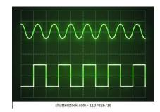
Identify an oscilloscope trace/signal as either analogue or digital.
