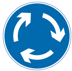
Mini roundabout (give way to traffic from the right)
