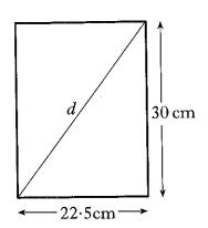
To check that the frame is rectangular, the diagonal, d, is measured.
