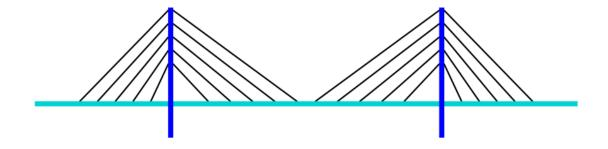
In a *fan* design, the cables all connect to or pass over the top of the tower(s).
