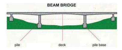
The downward force of the bridge's weight is supported by the ground. If the gap is too wide to be spanned by a single beam piers might be built at intervals to support a number of beams laid end to end.
