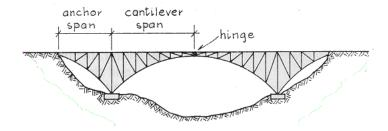
In cantilever construction, long rigid sections are used just like in a beam bridge. But instead of being attached to the river bank it is attached to cantilevers.
