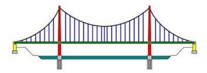
To take the strain, the ends of the cables are anchored in the banks. Old suspension bridges sometimes have chains rather than cables.
