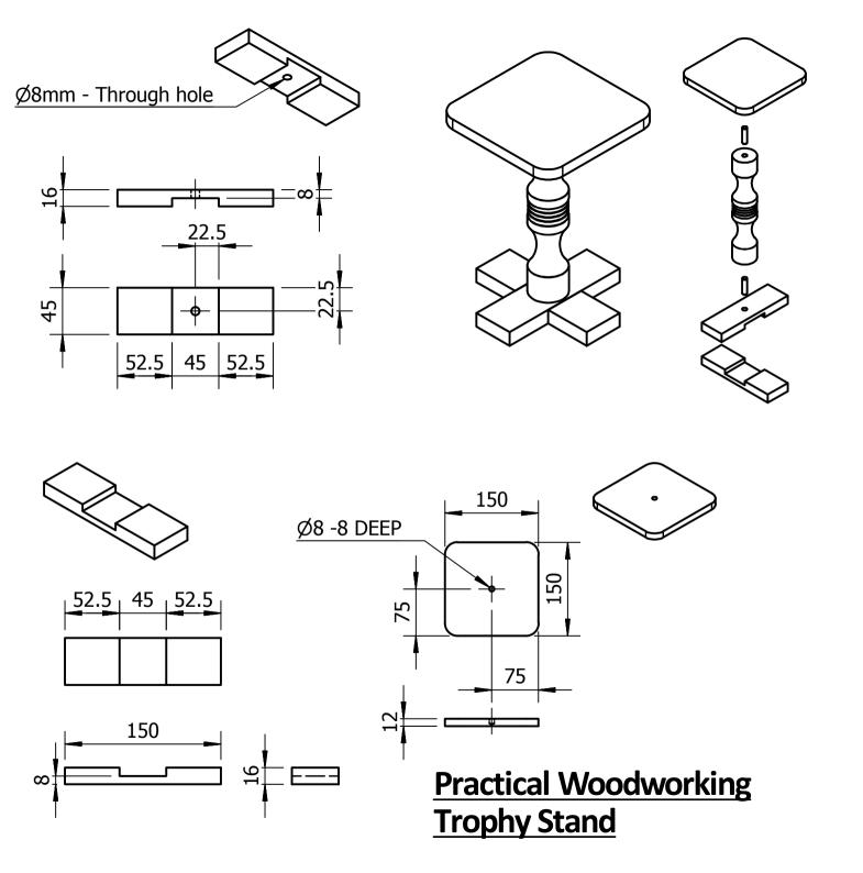
The blank is prepared for turning between centres on the woodwork lathe.
