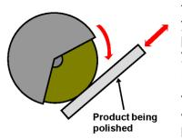
Always use the underside of the buffing wheel so that the product being polished is thrown away from you if it is pulled out of your hand. Never hold the product with a rag, it can catch in the wheel and drag your hand into the machine.
