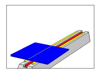
The third stage is to remove the soft heated acrylic and place it on a suitable JIG or FORMER.
