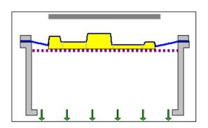
The final stage is to remove the pattern from the plastic leaving the finished article.
