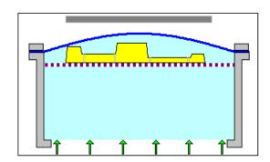
At this stage the air has been sucked out from beneath the plastic pulling it onto the pattern.
