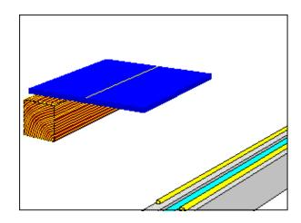
The last stage is to bend the acrylic to the desired shape.
