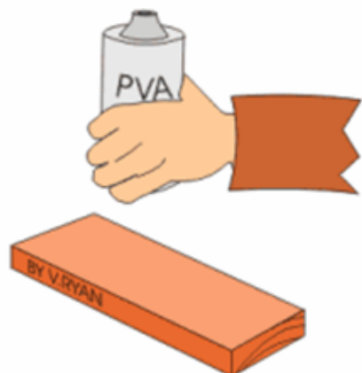
PVA GLUE APPLIED TO WOOD
