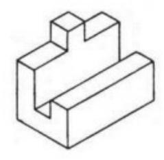
Shown is an isometric view of a complex shape. Your task is to put this shape into an *Orthographic*Sketch - ensuring you have elevation, plan and both end elevations completed.
