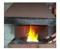
F\_\_\_\_\_ is used to heat up the metal prior to being worked on or finished.
