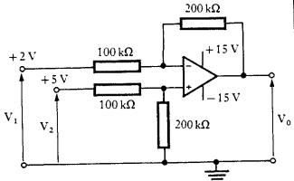
With the input voltages  $V_1$  and  $V_2$  as shown, what would be the output voltage  $V_0$ ?
