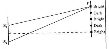
The figure also indicates the series of maxima and minima of intensity.
