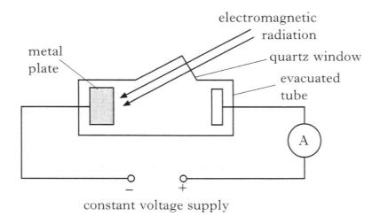
When light of wavelength 605 nm is incident on the metal plate, electrons are released with zero kinetic energy.
