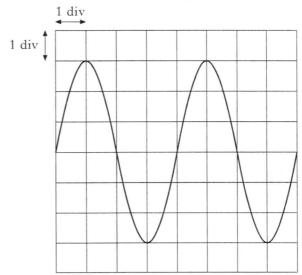
The time-base is set at  $0.01 \, \text{s/div}$  and the Y-gain is set at  $4.0 \, \text{V/div}$ .
