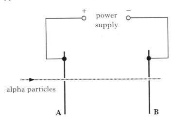
An alpha particle travelling at a speed of  $2.60 \times 10^6 \,\mathrm{m\,s^{-1}}$  passes through a hole in plate A. The mass of an alpha particle is  $6.64 \times 10^{-27} \,\mathrm{kg}$  and its charge is  $3.2 \times 10^{-19} \,\mathrm{C}$ .
