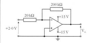
A voltage of  $+2.0\,\mathrm{V}$  is applied to the input. The voltage output,  $\mathrm{V_o}$ , is approximately
