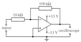
The input has a frequency of 280 Hz and a peak voltage of  $0.5\,\mathrm{V}.$
