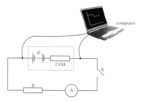
The computer connected to the apparatus displays a graph of potential difference against time.
