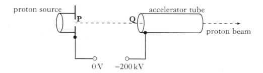
Protons released from the proton source start from rest at **P**. A potential difference of 200 kV is maintained between **P** and **Q**.
