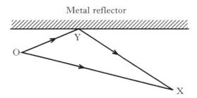
An interference pattern is produced.
