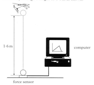
(a) The graph shows how the force on the ball varies with time during the impact.
