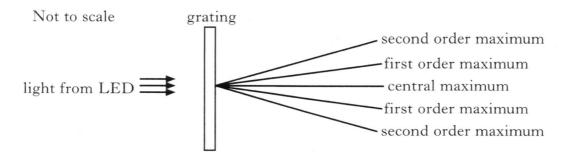
Light from this LED has a wavelength of  $6.35 \times 10^{-7}$  m. The spacing between lines in the grating is  $5.0 \times 10^{-6}$  m.
