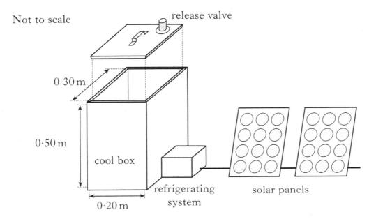
The lid is placed on the cool box with the release valve closed. An airtight seal is formed. When the lid is closed the air inside the cool box is at a temperature of 33 °C and a pressure of  $1.01 \times 10^5$  Pa.
