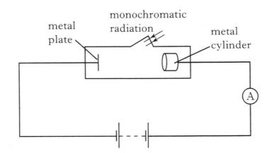
There is a constant potential difference between the metal plate and the metal cylinder.
