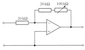
The variable resistor can be adjusted from zero to  $100\,\mathrm{k}\Omega$ . This allows the voltage gain to be altered over the range
