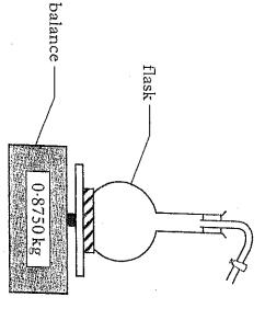
The air is now removed from the flask and the mass of the evacuated flask measured.
