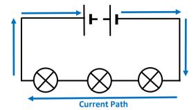
As you can see in the above diagram, the current path forms a continuous loop around the circuit.
