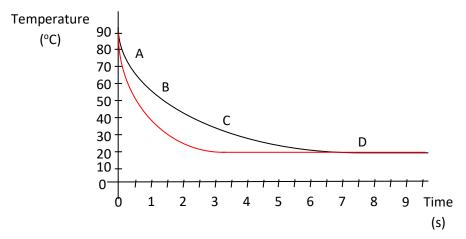
Heat loss is greatest at point \_\_\_\_A\_\_\_ on the graph. This is where the slope is the \_\_\_\_steepest\_\_\_\_\_.
