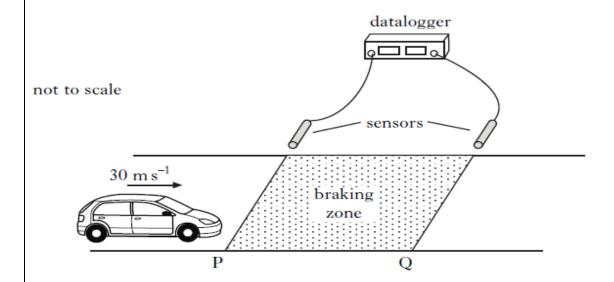
The sensors are connected to a datalogger which records the speed of a car at both P and Q.
