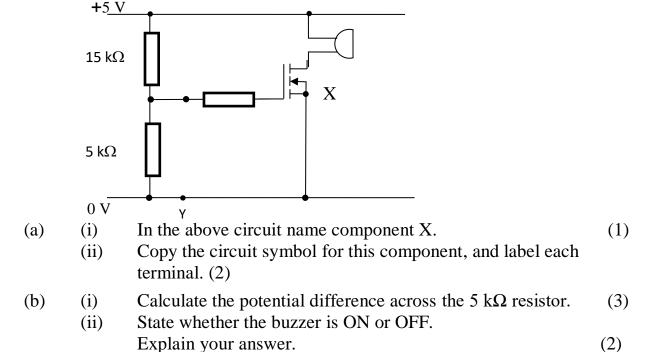
4. The circuit shown below is used as an alarm.
