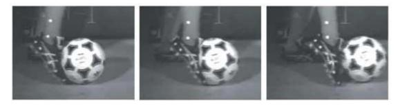
Once the foot makes contact with the ball a force is applied, the ball will compress as the force increases.
