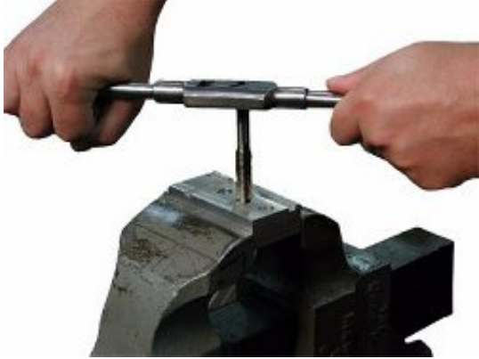
HOLE BEING TAPPED
