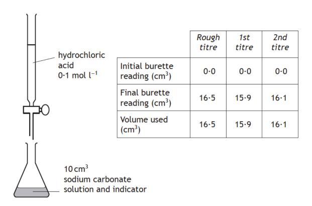
(a) Using the results in the table, calculate the average volume, in cm<sup>3</sup>, of hydrochloric acid required to neutralise the sodium carbonate solution.
