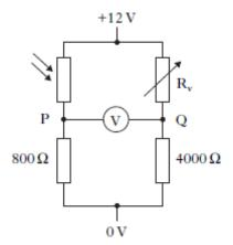
If the variable resistor,  $R_v$ , is set to  $6000\Omega$  and the LDR has a resistance of  $1600\Omega$ , what is the p.d. across the  $800\Omega$  resistor?
