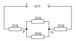
a) Calculate the total resistance of the circuit.
