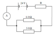
The reading on the ammeter is 2.0A
