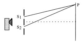
A microwave detector shows a minimum at P. P is the position of the first-order minimum, ie it is the second minimum from the centre.
