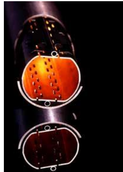
Cross-section of LHC prototype beam pipes showing the beam screens. Slits in the screens allow residual gas molecules to be pumped out and frozen to the walls of the ultra-cold beam pipe. Beam screens like these have been designed to line the beam pipes, absorbing radiation before it can hit the magnets and warm them up, an effect that would greatly reduce the magnetic field and cause serious damage
