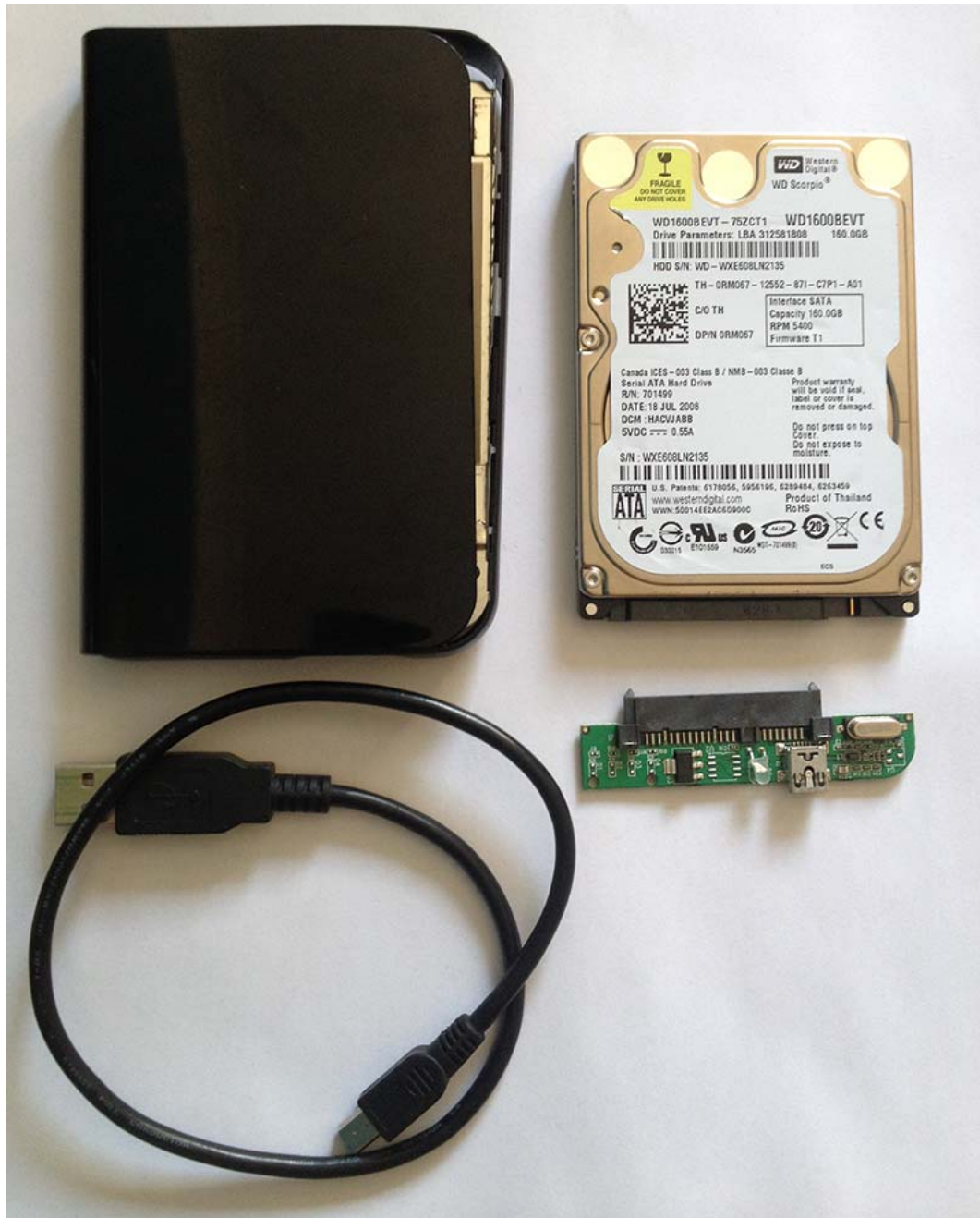
Figure 9.7: Parts of an external hard disk drive
