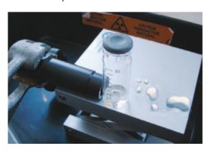
3) The half-life demonstration [11] with a Cs-137/Ba-137m Isotope Generator is permissible even although this source is an open source. The risk of harm that could result from the spillage of the eluate is trivial. Personal protective equipment to be worn during this demonstration are gloves and labcoat.
