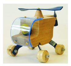
(a) The main body of the helicopter was manufactured by laminating two pieces of hardwood and one piece of softwood.
