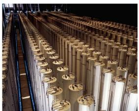
Fig. 20: Cascades of gas centrifuges in a US fuel enrichment plant in Piketon, Ohio.
