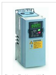
Fig. 4: The Vacon NX frequency driver (a.k.a. frequency converter). This device is controlled by the S7 PLC through a CP-342 module, and regulates accordingly the speed of the electric motor of the centrifuge to which is connected.
