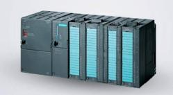
Fig. 1: The Siemens Simatic S7-300 PLC (CPU 315), equipped with a 24 V power supply and four I/O modular units. This is exactly the PLC model hunted by Stuxnet.
