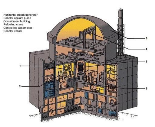
Fig. 21: The Russian VVER-1000 Pressurised Light Water reactor plant layout.
