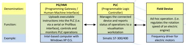
Fig. 2: block diagram of an ICS environment
