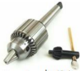
Jacobs chuck (3 jaw chuck) and chuck key
