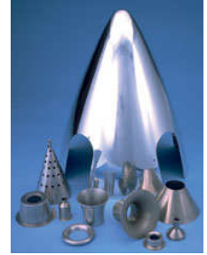
A selection of the sheet metal products that are manufactured by spinning.
