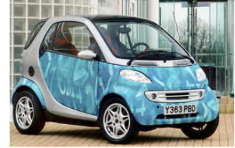
Aqua transfer printing used to apply the decorative finish to the body panels of the Smart car.
