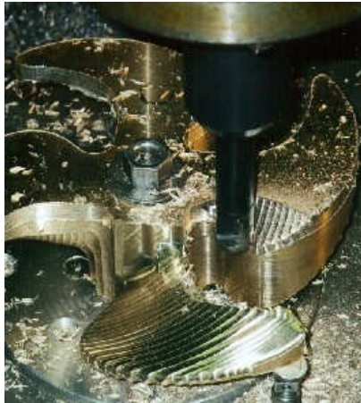
A boat's propeller being milled out of solid brass as an alternative to casting.
