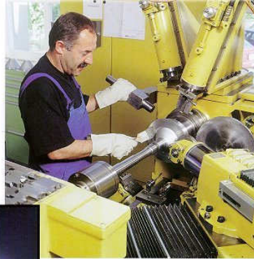
A sheet metal lampshade being formed by spinning
