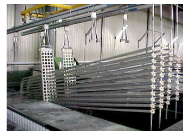
Anodised aluminium pipes removed from the electrolytic tank.
