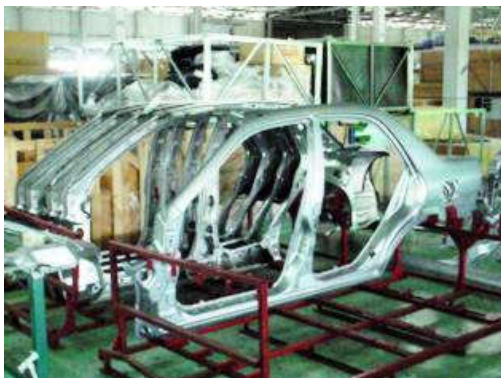
Mild steel car body panels: blanked, pierced and press formed ready to be spot welded together
