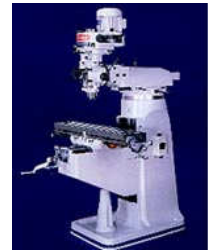
A manual milling machine used for one-off or low volume batch production.
