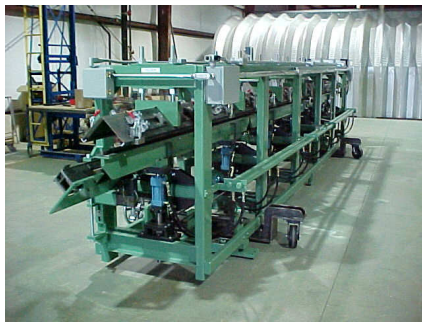
A press-forming machine used to produce simple bends on sheet metal used on building cladding.
