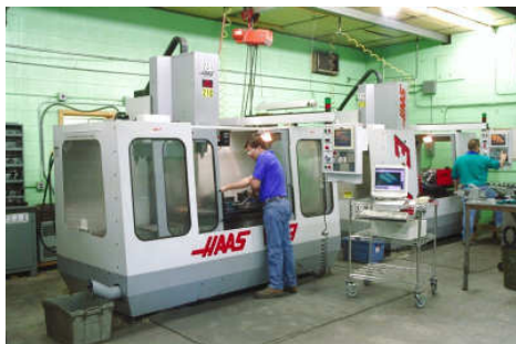
A CNC milling machine which uses the CAD drawing to generate the control program for the movement of the cutting tools.
