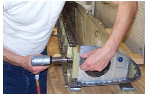
Pop rivets and an air operated pop rivet gun used to join sheet aluminium to an aircraft wing.
