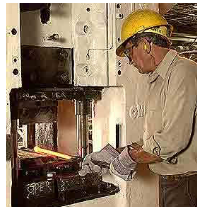
Power hammers being used to forge steel engine components.
