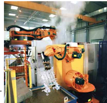
A robotic arm used in an automated factory to remove components after die casting.
