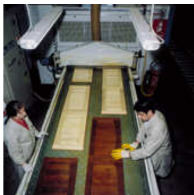
Line production and finishing of kitchen doors. This automated process involves the sanding, spraying and drying of the wooden components
