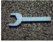
A simple steel spanner for use with flat-packed furniture is produced by blanking
