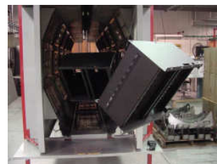
The cured powder coated components move out of the UV oven on the overhead conveyor.
