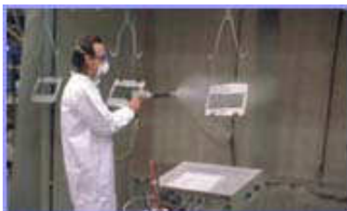
Electrostatic charged powder attracted to the oppositely charged component.
