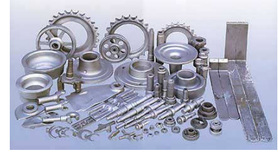
A selection dropped forged steel components.
