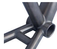
Titanium bike frame TIG welded together
