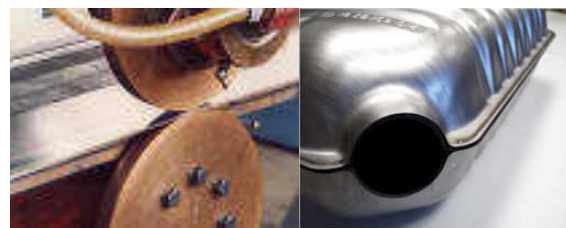
Seam welding where two round copper electrodes roll along the edge forming the weld. This technique is limited to products where the electrodes can follow the outside profile such as in the sheet steel fuel tank for a car.
