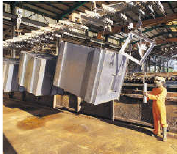
Galvanized steel bins being removed from the liquid zinc.
