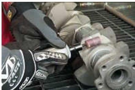
Hand finishing the flashing on a drop forged crank shaft for the diesel engine
