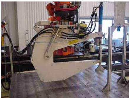
A robotic arm with a self-piercing riveter used for high volume production.
