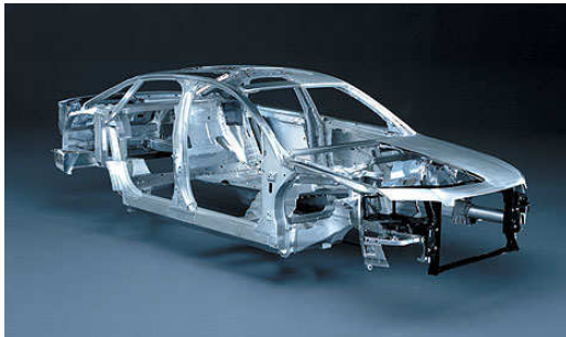
The aluminium space frame chassis for Audi's new A8 luxury car.
