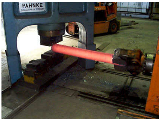
Power hammers being used to forge steel engine components.
