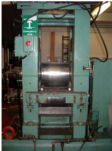
Rolling machine set up to produce rectangular bar or sheet.
