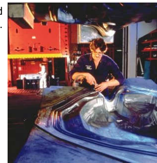
A complex 3D shape press-formed in stainless steel.
