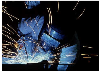
Manual Arc welding of steel.
