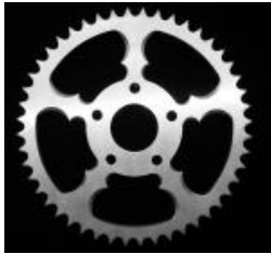
A bicycle sprocket is made in one operation by blanking (outer shape) and piercing (internal detailing)
