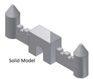
After making the computer 3D model, **generate orthographic views** for the production drawings. The generated orthographic views should include; centre lines, hidden detail and overall dimensions to aid manufacture.
