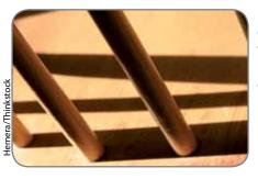
**Dowel rod** is circular sections of wood which can be bought in different diameters.
