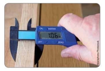
Tolerances provide the maximum (+) and minimum (-) deviation from the actual value that will still allow it to do its job.
