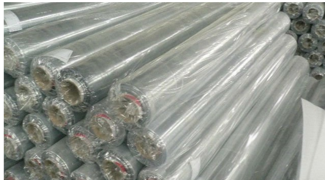
(above) PVC rolls produced by calendaring.
