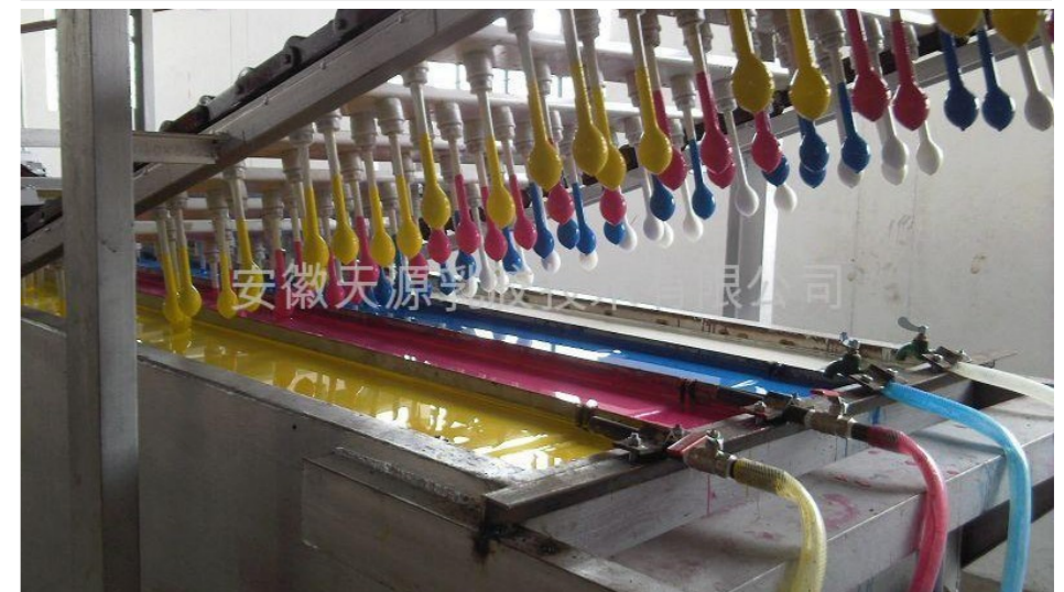
Balloons are mass produced using dip moulding.
