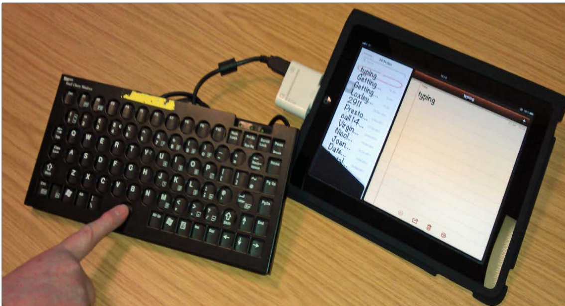
Figure 128: Example of a compact keyboard with keyguard using the USB.
