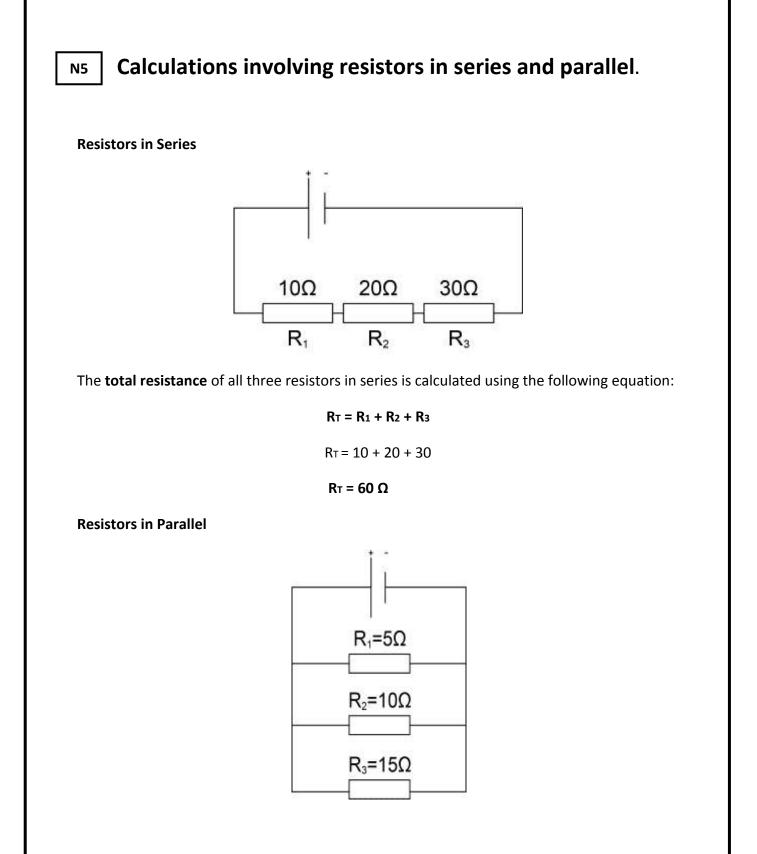
The **total resistance** of all three resistors in parallel is calculated using the following equation:
