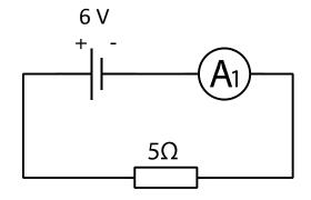
Calculate the value of current through the resistor.
