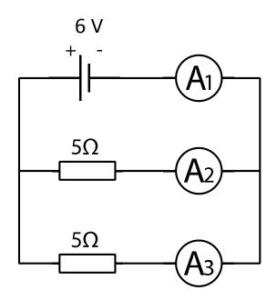
Calculate the value of the current through ammeter A1.
