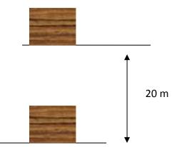
The 2 kg box has to be lifted up 20 m onto the shelf above it. The work done against gravity can be calculated using  $\mathbf{E_w} = \mathbf{F} \mathbf{x} \mathbf{s}$ .
