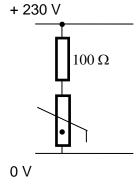
Calculate the potential difference across the thermistor when it is
