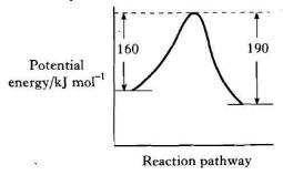
When a catalyst is used the activation energy of the forward reaction is reduced to  $35 \,\mathrm{kJ} \,\mathrm{mol}^{-1}$ .
