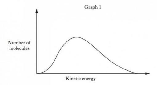
Add a second curve to Graph 1 to show the distribution of kinetic energies at 50  $^{\circ}$ C.
