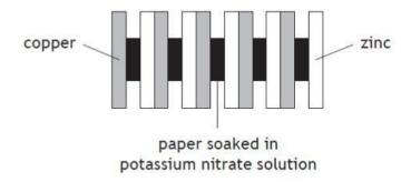
The purpose of the potassium nitrate solution is to complete the circuit. State the term used to describe an ionic compound which is used for this purpose.
