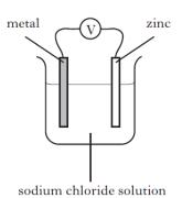
Which of the following metals, when linked to zinc, would give the highest cell voltage?
