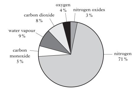
(a) What evidence in the pie chart shows that incomplete combustion of petrol has taken place?
