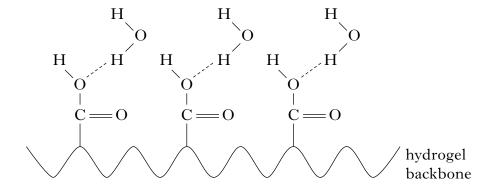
What type of bonding must be present **in the water molecules**, which allows them to be attracted to the hydrogel?
