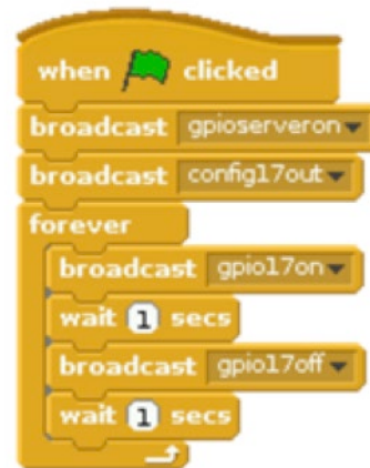
Figure 3.31 Scratch code to flash an LED connected to GPIO pin 17 on a Raspberry Pi. CC by-sa Raspberry Pi Foundation
