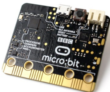
Figure 3.34 The other side of the BBC micro:bit showing power and data connectors, processor, accelerometer, compass and reset button
