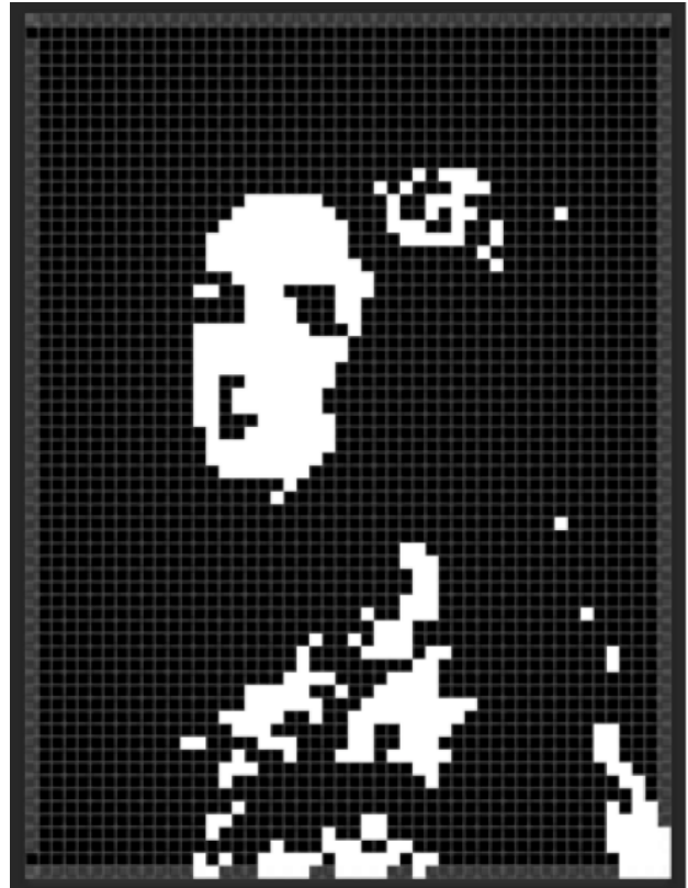
Figure 3.10 3,550 pixel bitmap, 1 bit per pixel, so 419 bytes of memory
