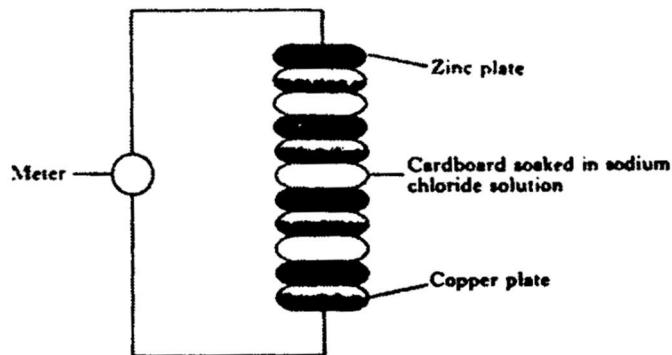
The Italian professor, Alessandro Volta, made one of the first batteries. It is called the “Voltaic Pile”. The diagram opposite shows the pile connected to a meter for measuring current.
