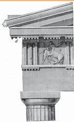
Doric Parthenon showing the top of a column, the entablature and frieze above, topped by a triangular pediment
