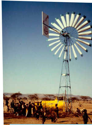
Wind turbine used to pump ground water in Kenya
