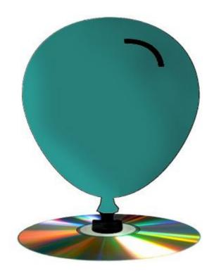
A hovercraft is also called Air-Cushion-Vehicle (ACV). It uses a blower to create air currents beneath itself. Resulting in the formation of air cushion that slightly lifts the craft upward. This upward lift reduces the friction of hovercraft with the surface on which it moves. Also, the lift allows it to move freely in any direction when pushed. We will build a model of hovercraft out of home materials, and this it will use the same principle.
