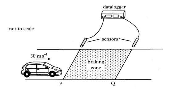
The sensors are connected to a datalogger which records the speed of the car at both P and Q.
