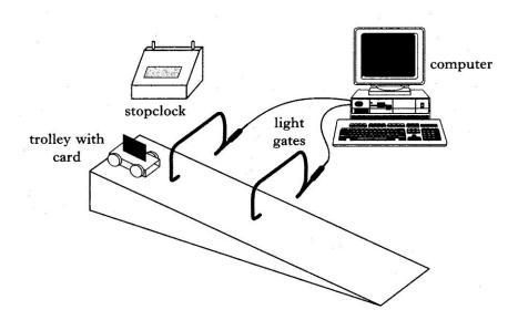
The trolley has a card mounted on it. As it moves down the track the card cuts off the light at each of the light gates in turn. Both the light gates are connected to a computer which is used for timing.
