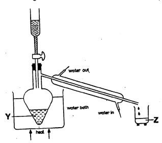
A student set up this apparatus in an attempt to prepare a few ml of reasonably pure propanoic acid by the oxidation of propan-1-ol. The latter was slowly introduced into the hot solution Y. The following information is available:
