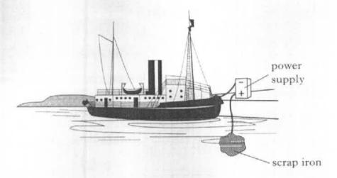
(a) (i) Why does connecting the ship to the negative terminal of the power supply prevent the iron in the ship from rusting?
